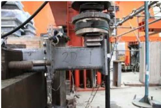
(c) Segment 1 connection before loading
