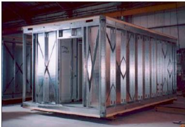
Fig 9. Continuously supported module in light steel framing
